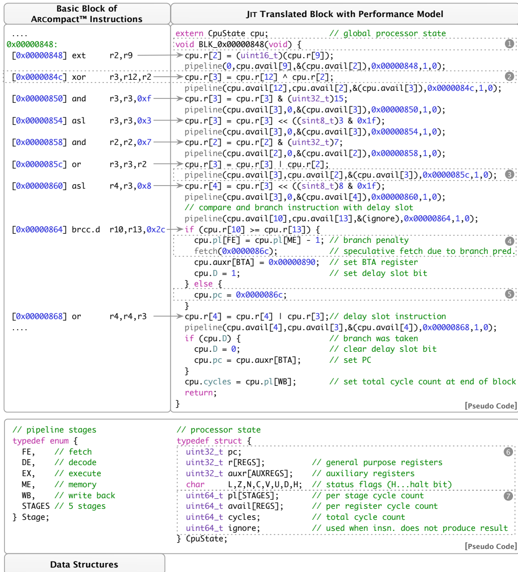
Figure 5.2: Dynamic binary translation of ARCompact basic block with CpuState structure representing architectural ⑥ and microarchitectural state ⑦. See Figure 5.4 for an implementation of the micro-architectural state update function pipeline() .
